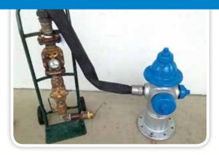
Secure and transport meters safely; never leave unattended. Use OUC-approved fire hydrant wrenches (available in OUC's Water Meter Shop). FLUSH FIRE HYDRANT UNTIL WATER IS CLEAR BEFORE ATTACHING PORTABLE WATER METER. Install assembly in vertical upright position. Operate in horizontal position (with dial facing up).
