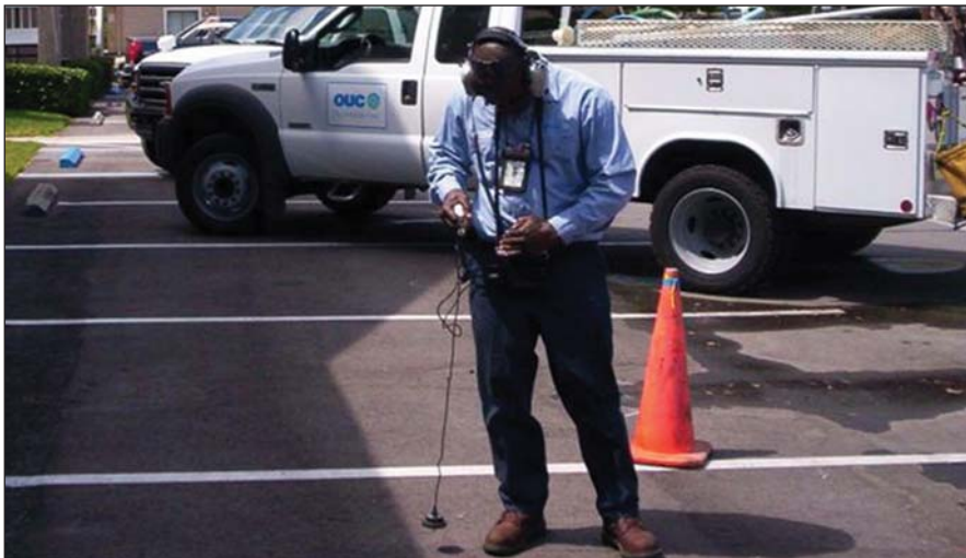
Benny Florvil uses special equipment to locate leaks in underground water pipes.
